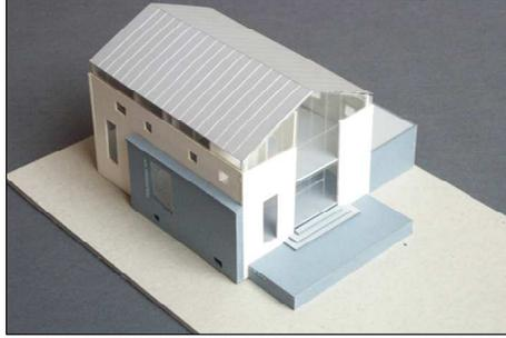
The walls of a single storey A-frame house are to be extended upwards to create a full two-storey house for the family of a stone mason. The existing walls of the ground floor and garage that are original will have their render removed and be clad by the owner with pieces of stone. All new walls will have a white render finish, thus delineating old from new.
