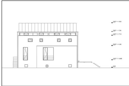
A new band of clerestory windows separates the walls from the new roof, providing all rooms with ample daylight while protecting the privacy of the family. The entrance has been moved from the east side to the front, nearer to the garage for convenience.
